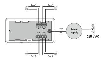
To connect the control unit to the fan units, a 3-pin plug must be connected to the cable. The plug must be wired as shown below.
