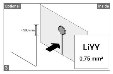
Lay the cables for a decentralised home ventilation system (to be installed at a later date) via slits in the wall / cable ducts up to the installation cylinder. Make sure that at least 300 mm of cable protrudes, enabling the units to be connected up. Further details are to be found in the installation instructions for the corresponding ventilation unit.
