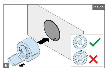
Open the calculated number of chambers for the sound insulation elements. Carefully take out the pre-cut parts and insert the right number of them into the installation cylinder, making sure that the opened chambers all point in the same direction.
