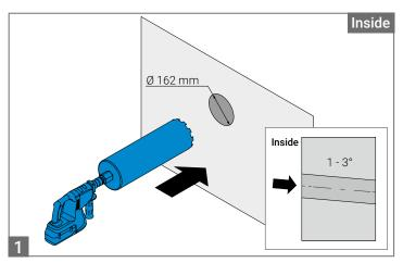
Core-drill a hole (Ø 162 mm) in the outside wall or use a pre-fabricated installation block. The hole must have a gradient of 1-3° towards the outside
