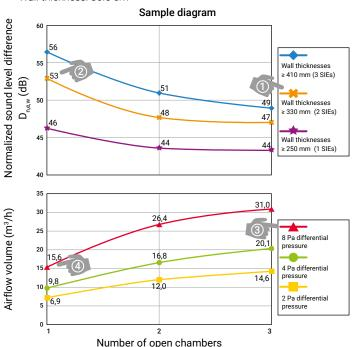
» 8 Pa differential pressure through the use of a centrifugal fan in the bathroom
