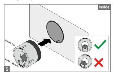
Insert the wind pressure protection into the installation cylinder. Make sure that the unit with the pre-filter is inserted first. The wording "OBEN  $\uparrow$  TOP" must point upwards, while the wording "INNEN / INSIDE" must point inwards.
