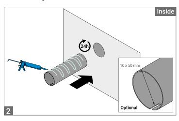
Measure the wall thickness, taking account of any future plastering. Please also pay attention to the installation instructions for the selected outside vent cover / special solution. Cut the installation cylinder to the required length.
